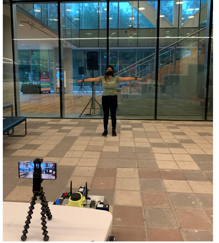
Fig. 4: Example of set up, with a cellphone's camera mounted on a tripod and Intel D435i camera, calibration phase's pose is being done by the current subject.
